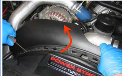
3. Loosen the upper hose clamp at the OE elbow and pry the compression clip out of the groove.
