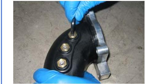
8. Install the OE O-ring from step #5 into the groove in the base of the S&B Elbow.
