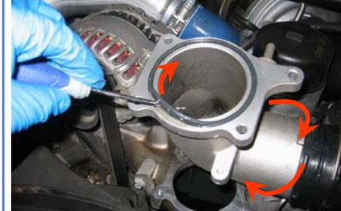
6. Remove the OE elbow from the boost tube. Careful not to let any debris fall into the intake manifold or the boost tube.
