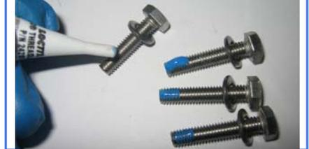
11. Thread the bolts by hand into the intake manifold to secure the S&B Elbow. Torque the bolts to 100 In. lbs. If you use a 10mm crow foot to torque the bolts under the bend. See the crow foot torque wrench calculation on page 2.
