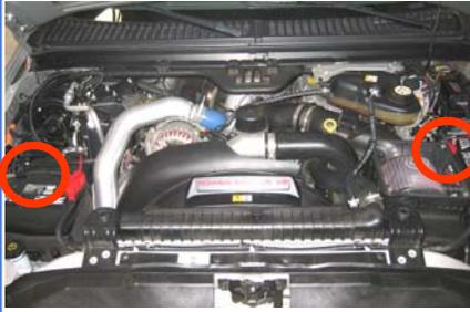
2. This step is **optional** and will only allow you better access to the elbow mounting bolts. Use a small flat head screwdriver and pry the clips open and pull up working your way across to remove the upper fan shroud.
