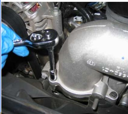
5. Rotate the elbow and remove the rectangular O-ring. Wipe clean and set aside. Careful not to let any debris fall into the intake manifold.
