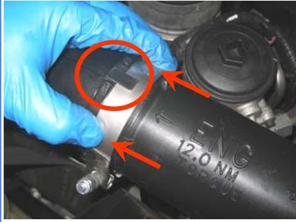
14. Align the upper fan shroud and snap into place.
